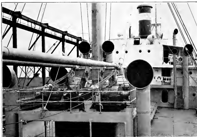
Cargo winches on the motorship City of Elwood, showing neat, elevated platform and enclosed deckhouse for resistors and contacts.
